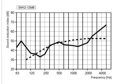
Diagrams shows sound reduction with fully opened diffuser and 300mm wall. Calculating on 10m<sup>2</sup>.
